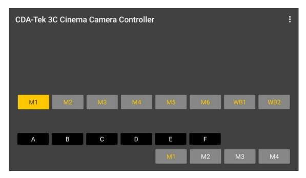
The Image presets (labelled M1-M6) store ISO, Aperture, Shutter Angle, White Balance Temperature and White Balance Tint.
