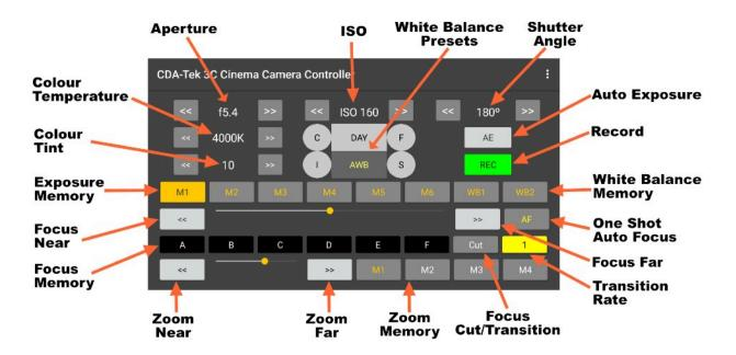
Within each block, there are also controls for the storage and recall of user presets for these functions.
