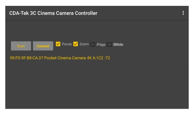
Pressing the "Scan" button will then present you with a list of Bluetooth LE devices and you should then press to select your camera from the list and then press the "Connect" button.
